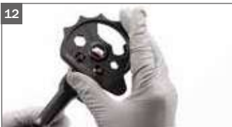
Align the air nozzle with the universal wrench (optional)
