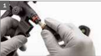
First remove paint needle.
