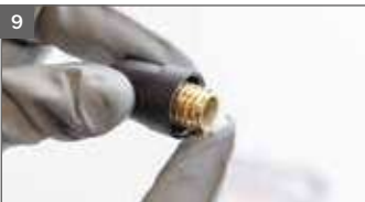
Grease thread of material flow control screw
