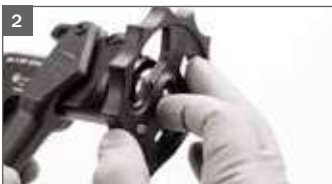
Tighten fluid tip by hand using the universal spanner.
